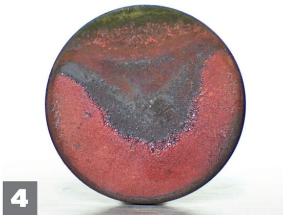
**4** **GREEN MEANS STOP.** The green area at the top shows this **valve should be replaced immediately.** (Note how the uneven burn patterns match the heat distribution chart.)
