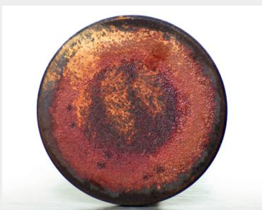
Don't be alarmed by the bright color, or deposits around the edges. The symmetrical pattern shows this valve is just fine.
