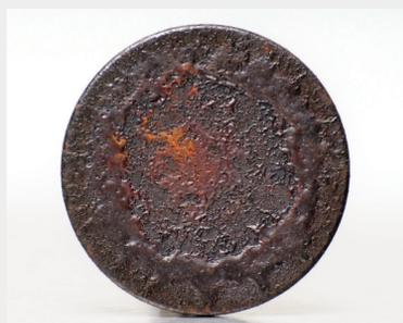
Thick lead deposits from an overly rich mixture give this healthy valve the appearance of an overcooked pizza.
