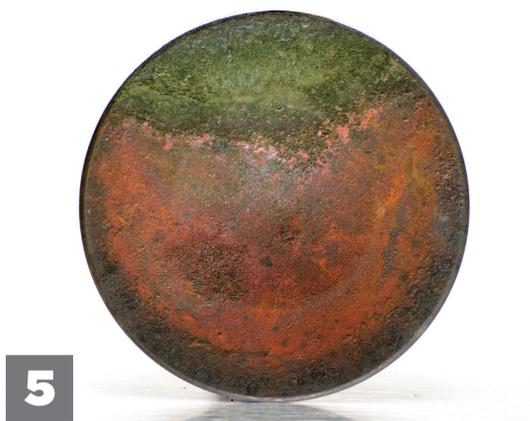
**5** Green crescent progresses toward center with valve cracking and failure a serious danger.
